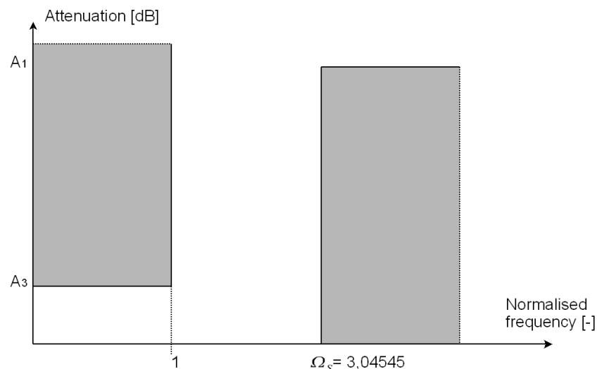
Calculate the L and C components of the Chebyshev low-pass filter. The topology with two parallel capacitors and one series inductor is chosen. The resistor  $R_s$  of the voltage source is equal to 1 Ohm.
